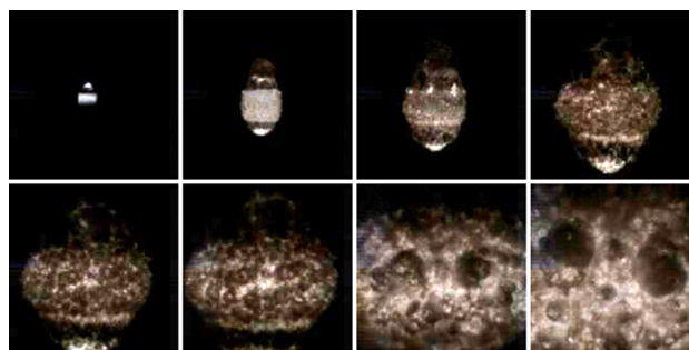
Fig. 12 Prompt fragment reactions upon detonation from a cylindrical 1 kg C4 charge in a 73.5 mm inner diameter, sintered Zr casing ( M/C = 1.85 )
