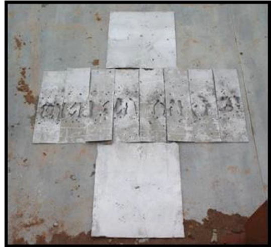
FIG. 5—Aluminum witness panels from recovery packs.
