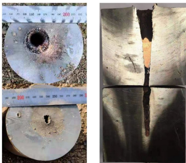
Figure 11. Experimental results of the copper jet against the steel target (on the left is the entrance hole view of the steel plates; on the right is the section view of the steel plates).
