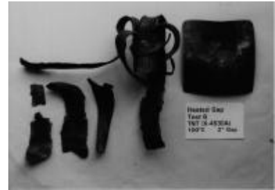
HGT-6. TNT, 2-inch gap, 100°C.
