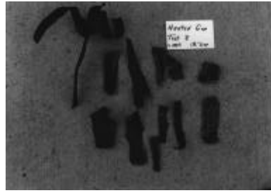
HGT-8. TNT, 1.5-inch gap, 100°C.
