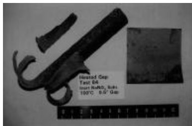
HGT-84. Inert, 0.5-inch gap, 100°C.
