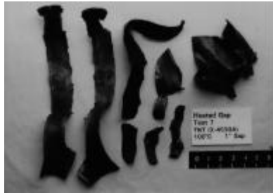
HGT-7. TNT, 1-inch gap, 100°C.
