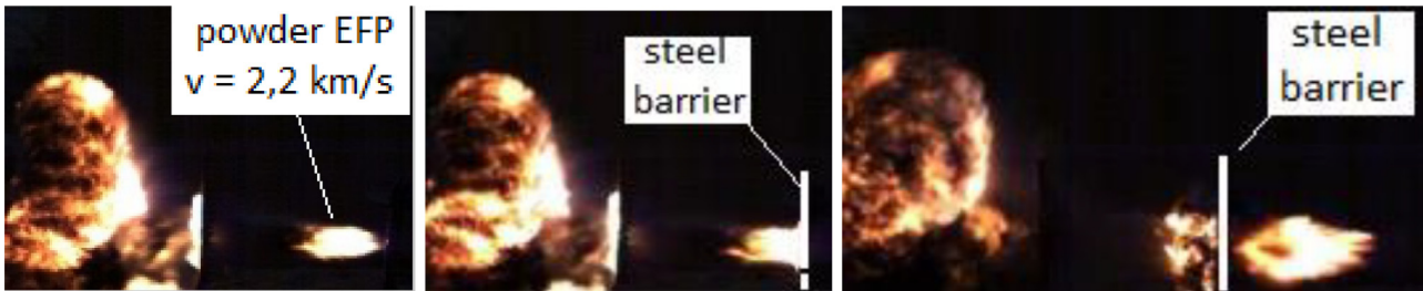
Fig. 5. Images taken with high-speed camera show EFP in flight after time 250 μs (first image), at the moment of hitting a steel barrier after 300 μs (second) and after penetration of a barrier (400 μs). Time is counted from a moment of a cap detonation.
