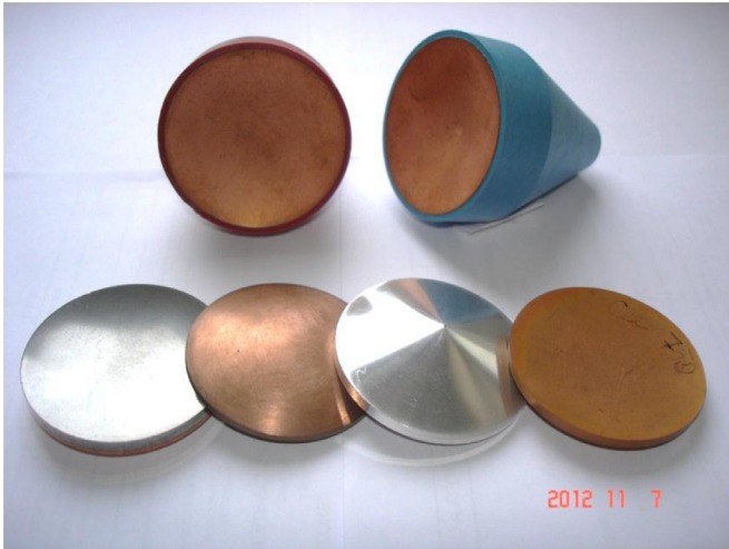
Fig. 1. Spherical liners made of different metal powders and EFP charges (at the top) with different sintered metallic powder liners.
