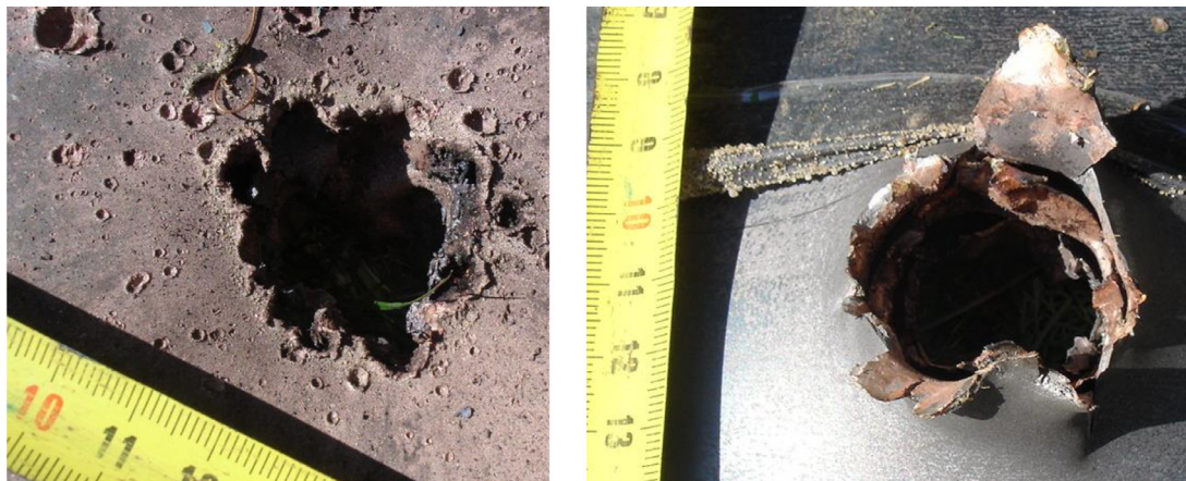
Fig. 6. Pictures showing a 15 mm (3 × 5 mm) thick steel barrier penetrated by a copper powder EFP that was initiated at a distance of 1 m. Inlet of a projectile (left) and outlet (right).
