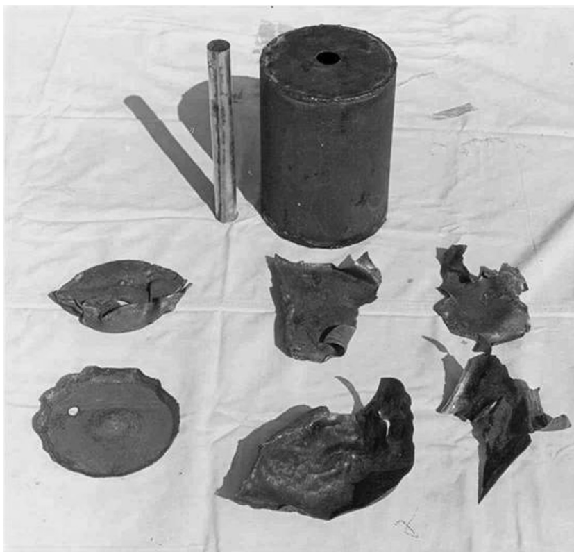
Fig. 3. Fragments obtained from breaking of un-serrated canister using NQ burster charge.
