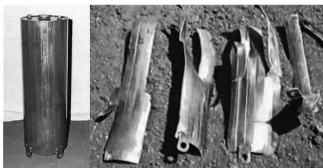
Figure 6. Canister with 2.95 H/D and the according fragmentation pattern (burst charge: 143 g NQ, burst charge loading: 0.32 \text{ kg m}^{-2} ).
