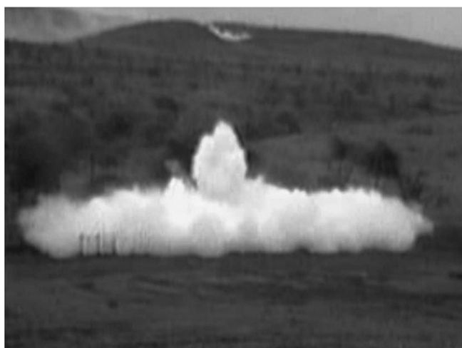
Figure 7. Aerosol formed for a canister with 1.5 H/D (fuel: 18.5 kg propylene oxide, burst charge: 120 g NQ, aerosol height: 2.05 m, diameter: 19.4 m, H/D: 0.10).
