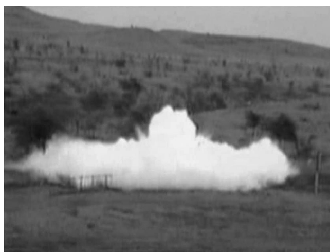
Figure 8. Aerosol formed for a canister with 2.95 H/D (Fuel: 18.5 kg propylene oxide, burst charge: 143 g NQ, aerosol height: 2.5 m, diameter: 13.3 m, H/D: 0.19).
