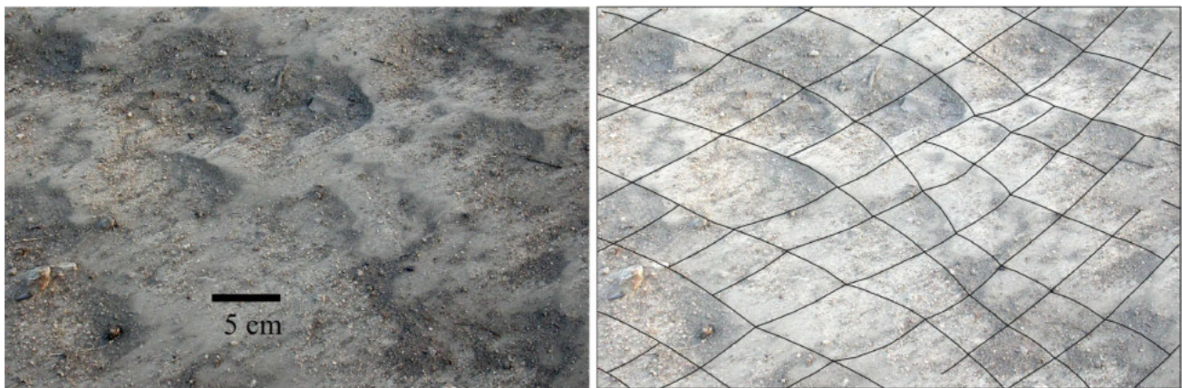
Fig. 7 A fine-soiled particle ground record produced by gasoline spray detonation propagating from left to right ( left ) and the authors' interpretation of the cellular structure ( right )
