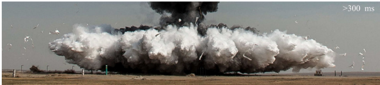
Fig. 11 Explosive dispersal of 5,100 kg gasoline: liquid fracture, fragmentation and jet formation
