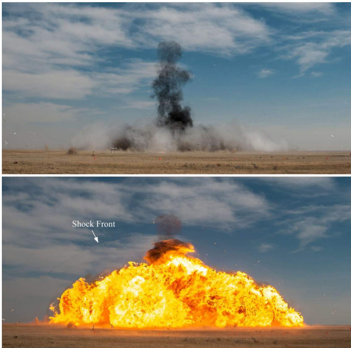
Fig. 3 Photographs before and after detonation of dispersed gasoline spray cloud
