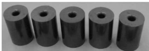
Figure 2. 50 g charges of RDXph/Al-Mg.
