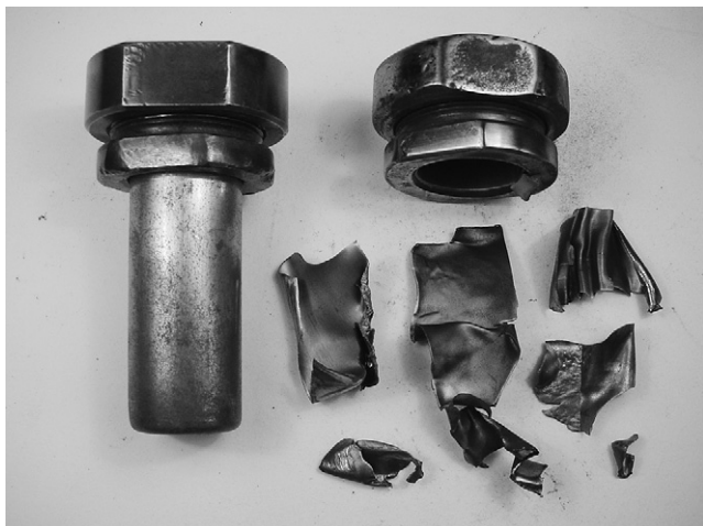
Fig. 2. Koenen test on DIAD at 1 mm (fragments > 7).
