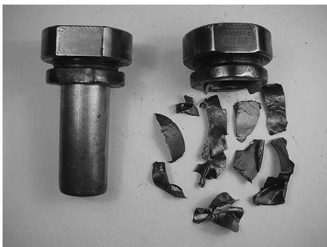
Fig. 1. Koenen test on DEAD at 20.0 mm (fragments > 9).
