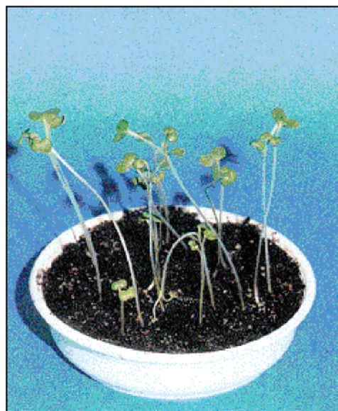
FIGURE 9. White mustard on day 21 after spraying with extract from the soil that had subjected to detonative decomposition of DNOC.
