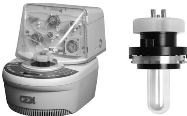
Figure 3.14 The CEM Voyager SF and its 80 mL reaction vessel.
