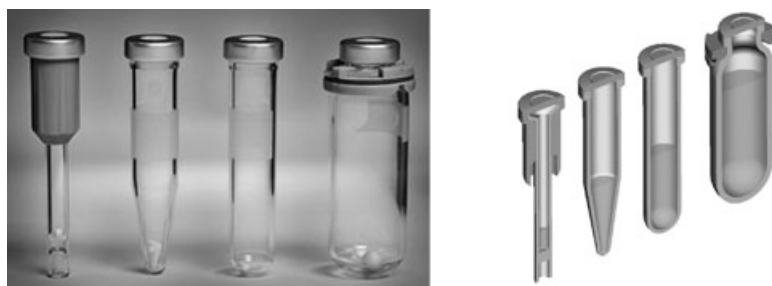
Figure 3.8 Biotage Initiator vessel types (0.2–0.5 mL, 0.5–2.0 mL, 2.0–5.0 mL, 10.0–20.0 mL, left to right) and schematic description of maximum volume.
