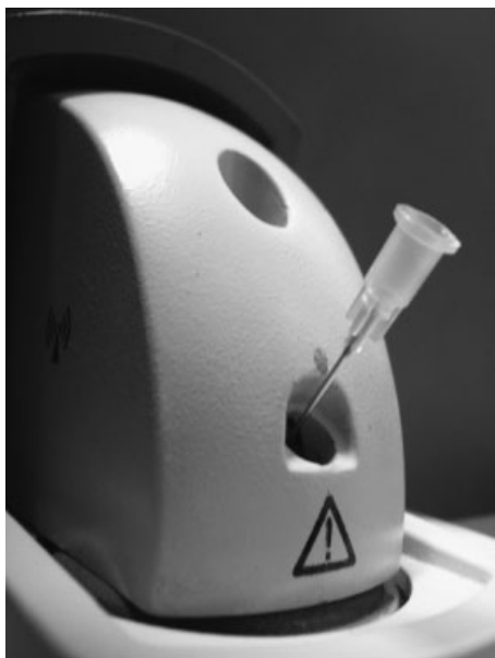
Figure 5.9 Overpressure release after the reaction (Biotage).
