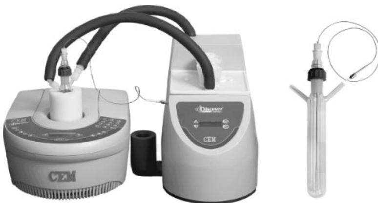
Figure 3.12 CEM Discover CoolMate: low-temperature cooling module.
