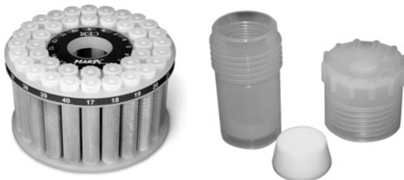
Figure 3.28 CEM MARSXpress rotor: Xpress 55 mL and screw-cap vial.
