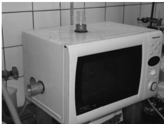
Figure 3.3 Modified domestic household microwave oven. Inlets for temperature measurement by IR pyrometer (left side) and for attaching reflux condensers (top) are visible. A magnetic stirrer is situated below the instrument.
