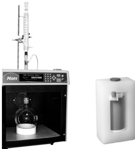
Figure 3.25 CEM MARS scale up systems: open vessel round-bottom flask with reflux condenser and high-pressure 300 mL vessel.
