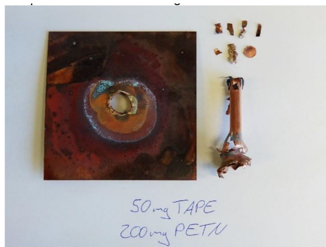
Figure 10. Positive initiation capability test of TAPE on PETN.
