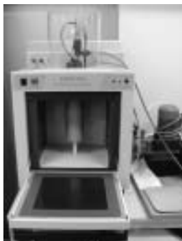
Figure 9.5 Commercial embodiment of the continuous microwave reactor (by Milestone MLS).
