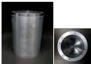
Figure 2. Final laminated casing after compaction by explosively compressed water and machining.
