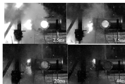
Figure 4. High-Speed Video of Experiment No. 4 with a Violent Reaction.
