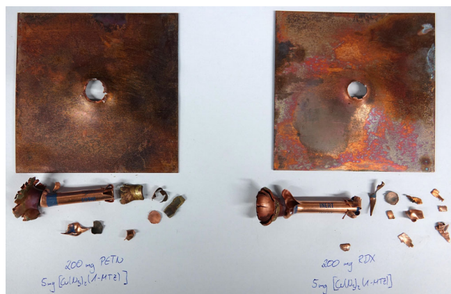
Figure 4. Positive PETN (left) and RDX (right) initiation tests with 5 mg of the coordination compound 1 .
