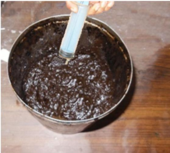
**Fig. 1** Injection of gassing agent to emulsion explosive
