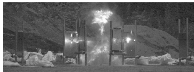
Figure 8. Image of ETN explosion obtained 1.2 ms after ignition. The moment that metal fragments hit the steel plates is shown. Bright sparks are observed after the impact.
