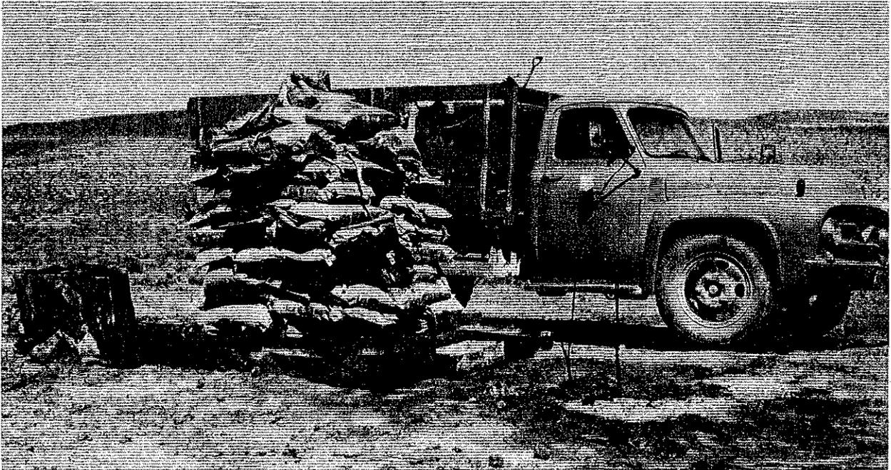
FIGURE 25. - Arrangement of 4,910 Pounds of Mixed AN, Paper Bags, and Urea. The urea content is about 12 percent.
