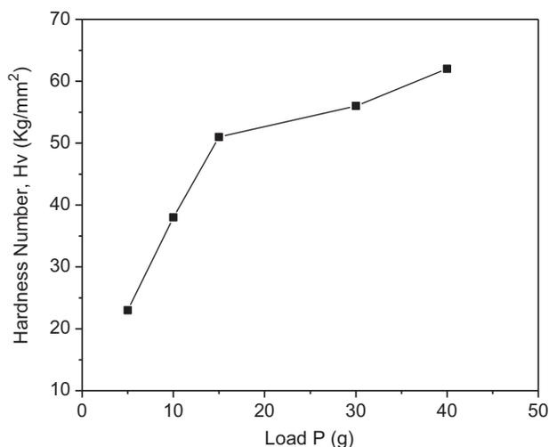
Fig. 8. Hardness number (Hv) versus load (P) of GPCl.
