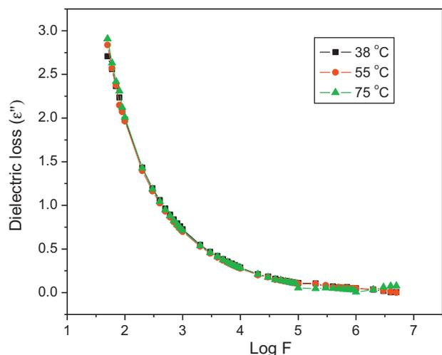
Fig. 7. Variation of dielectric loss with frequency of the applied electric field.
