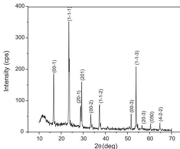
Fig. 2. X-ray powder diffraction pattern of GPCI.
