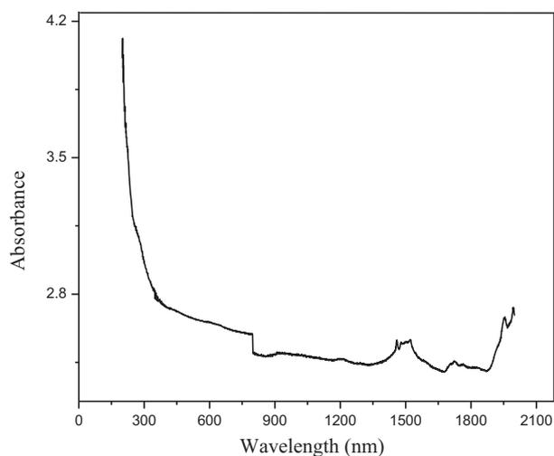
Fig. 4. UV-vis-NIR absorption spectrum of GPCI.
