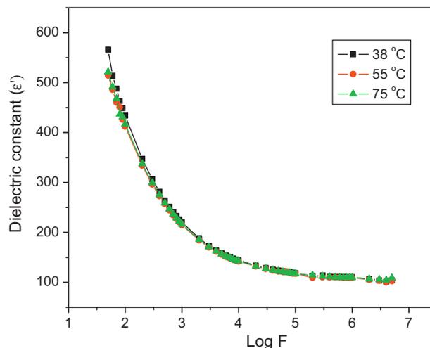
Fig. 6. Variation of dielectric constant with frequency of the applied electric field.
