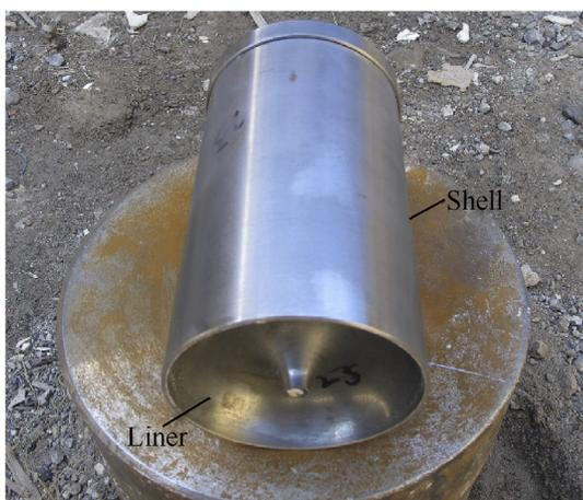
Fig. 1. The structure of a bore-center annular shaped charge.
