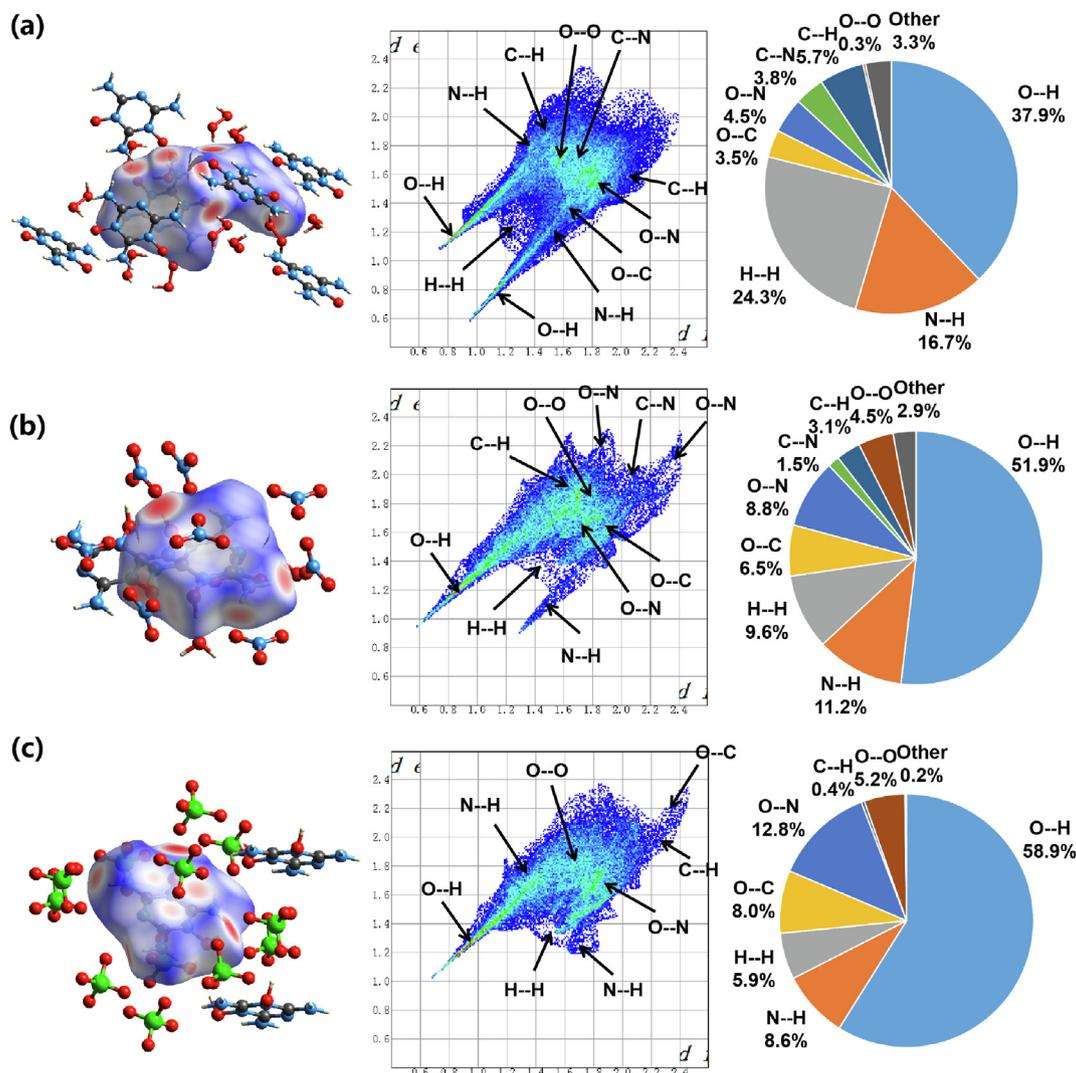
**Fig. 4.** (a) Hirshfeld surfaces, 2D fingerprint plots and the individual atomic contact percentage contribution of TTDH; (b) Hirshfeld surfaces, 2D fingerprint plots and the individual atomic contact percentage contribution of TTDON; (c) Hirshfeld surfaces, 2D fingerprint plots and the individual atomic contact percentage contribution of TTDOP.
