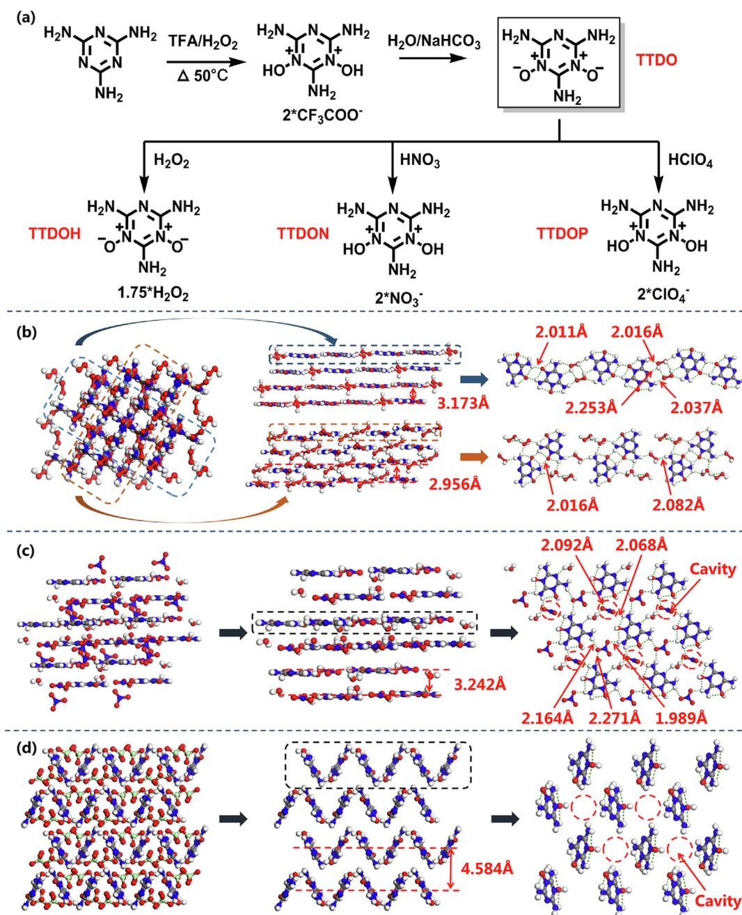
**Fig. 3.** (a) Synthesis routes of TTDO and the corresponding explosive-oxidant self-assembled energetic materials (TTDOH, TTDON and TTDOF). (b) 3D crystal structure and step-by-step enlarged view of TTDOH. (c) 3D crystal structure and step-by-step enlarged view of TTDON. (d) 3D crystal structure and step-by-step enlarged view of TTDOF.
