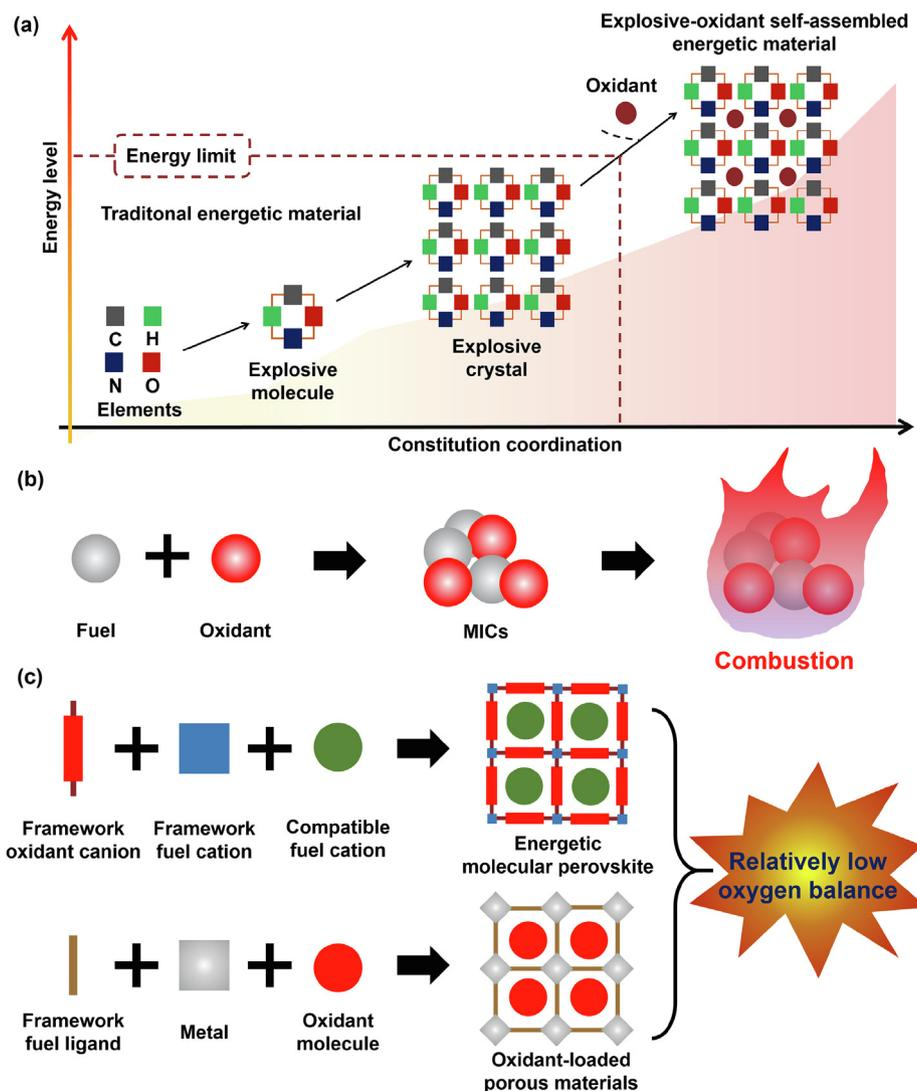
Fig. 1. (a) Illustration of explosive-oxidant self-assembled strategy and its comparison with traditional energetic material. (b) Schematic of metastable intermixed composites. (c) Schematic of energetic molecular perovskite and oxidant-loaded porous materials.
