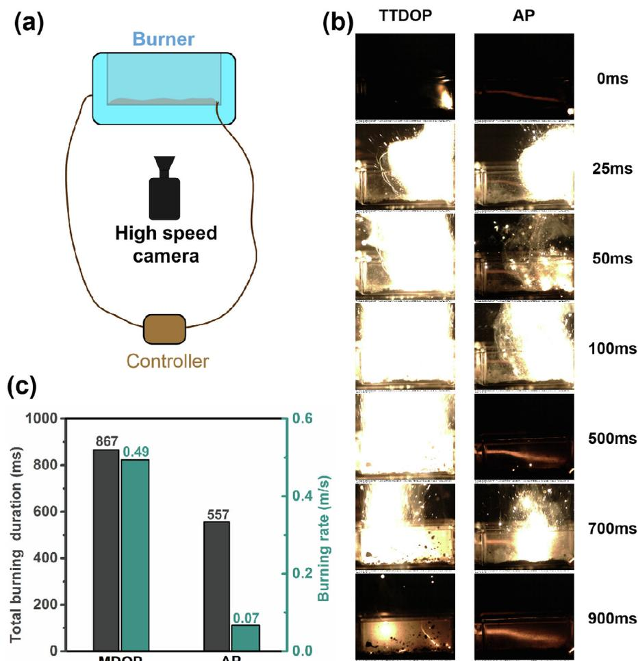
Fig. 5. (a) Schematic of combustion test device. (b) Combustion snapshots of TTDOP-Al mixed sample and AP-Al mixed sample. (c) Total burning duration and burning rates of TTDOP-Al mixed sample and AP-Al mixed sample.
