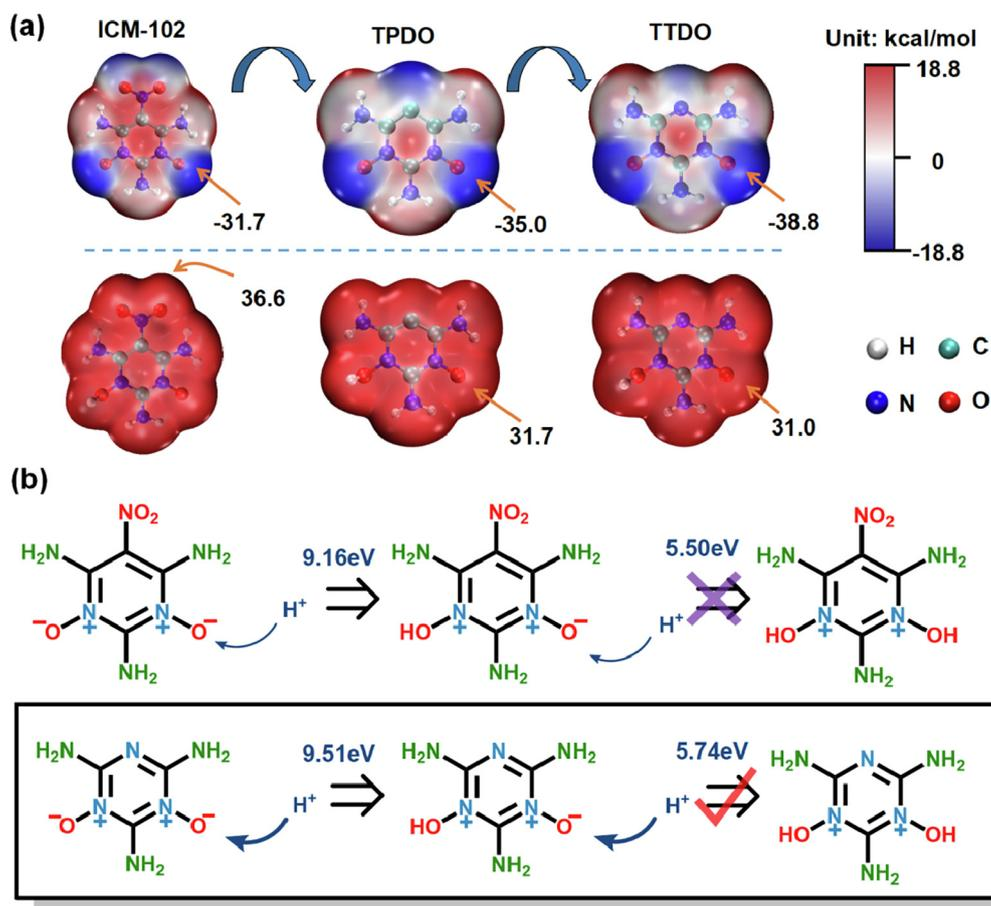
Fig. 2. (a) Electrostatic potential (at 0.001 a. u.) of ICM-102, TPDO and TTDO and their protonated derivatives. (b) Stepwise proton affinities for ICM-102 and TTDO.
