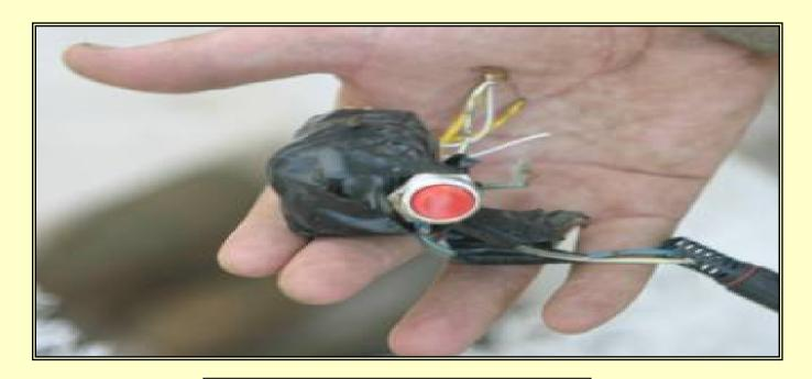
MANUAL TRIGGER FOR AN IED; CAN BE FOR A SUICIDE VEST IED OR SUICIDE VEHICLE BORNE IED
