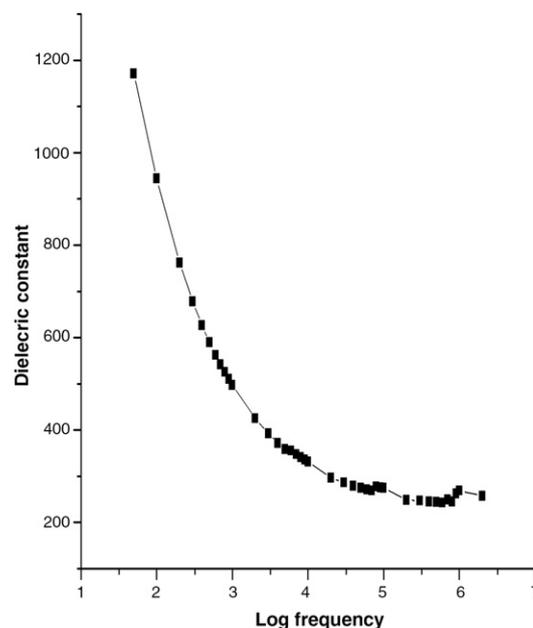
Fig. 6. Variation of dielectric constant of GLN with log frequency.
