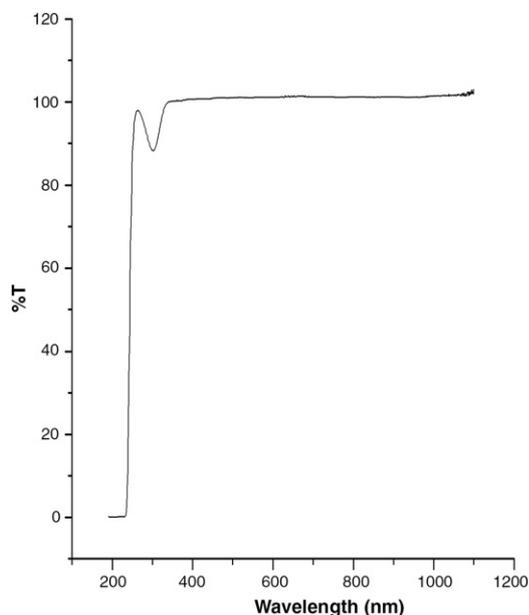
Fig. 5. Transmission spectrum of GLN.
