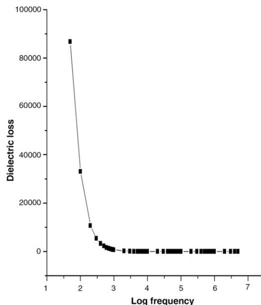
Fig. 7. Variation of dielectric loss of GLN with log frequency.
