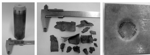
Figure 2. Picture of the UHP charge (36×100 mm) with HMX booster, in a copper tube, prior to detonation (left); fragmentation of the copper tube after the detonation (middle) and stainless steel witness plate after the explosion of the charge (right).
