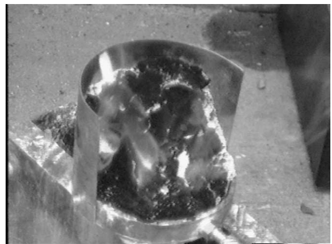
Fig. 3. Baby milk powder burning nest, burning mode—flame.
