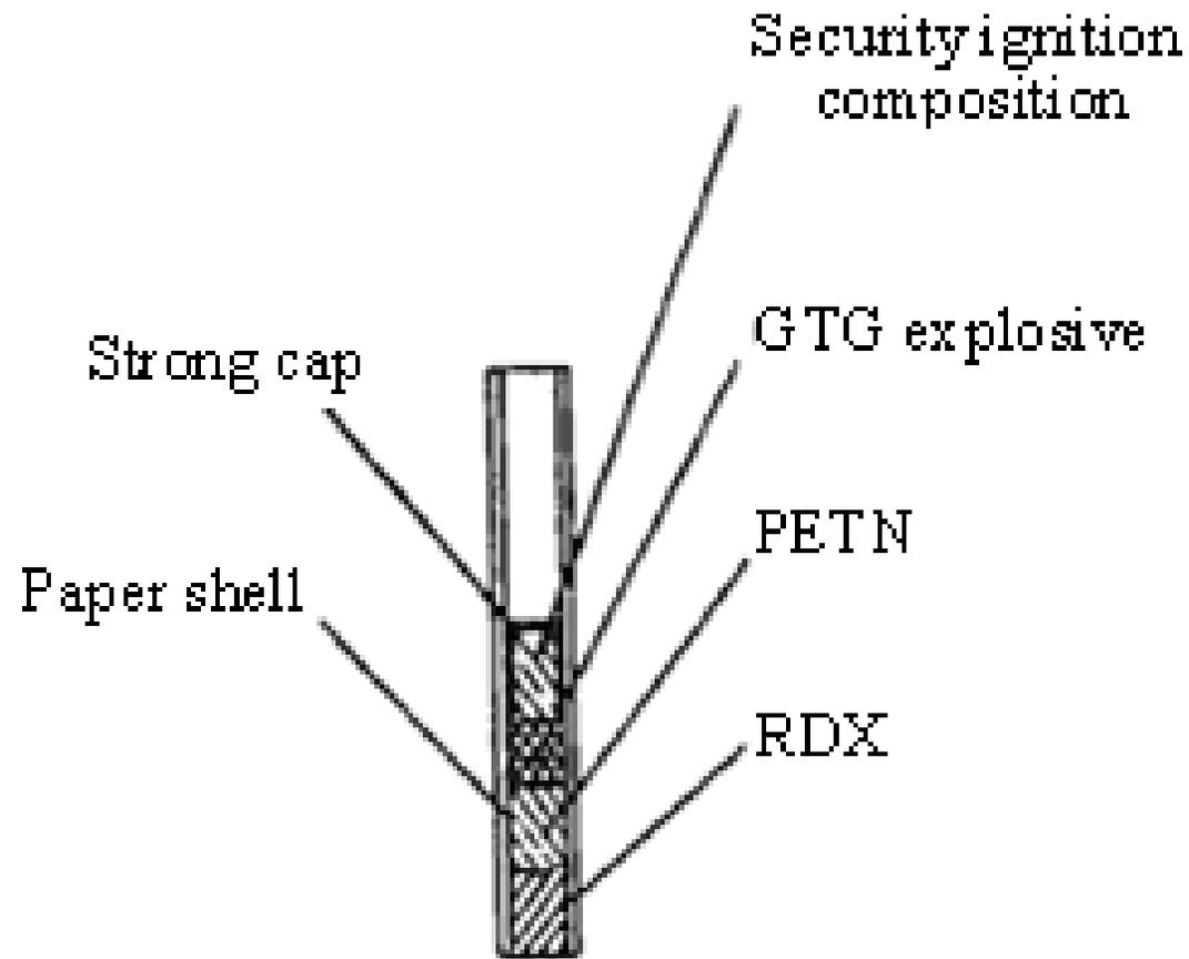
The structure of flame detonator with GTG
