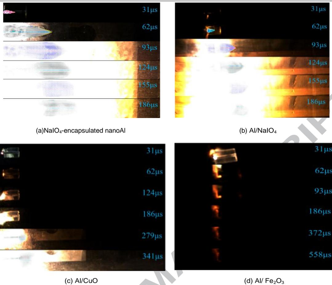
**Fig. 7.** Comparison of the reaction propagation in different proportions of (a)  $\text{NaIO}_4$ -encapsulated nanoAl and (b)  $\text{Al}/\text{NaIO}_4$ , (c)  $\text{Al}/\text{CuO}$ , (d)  $\text{Al}/\text{Fe}_2\text{O}_3$ .
