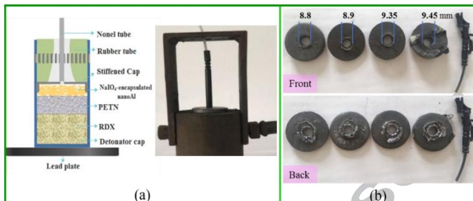
**Fig. 12.** Illustrations of (a) setup of explosive test and (b) results of the explosive test by lead plate method.
