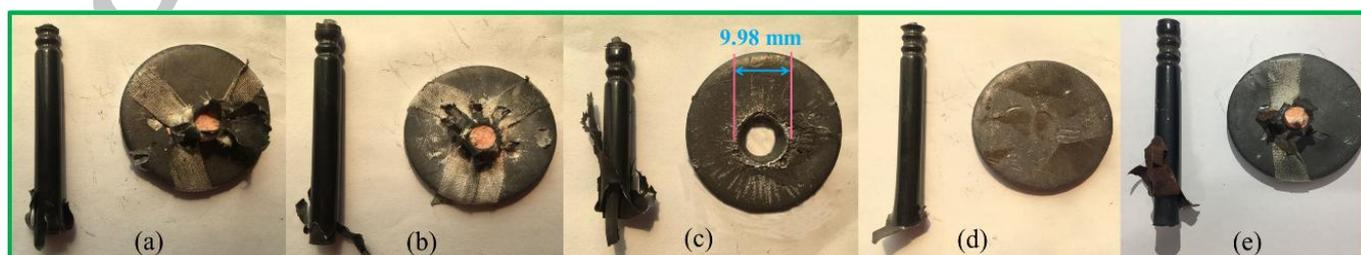
**Fig.13.** Illustrations of the results of detonation tests:(a)  $\text{Al}/\text{Fe}_2\text{O}_3$ ; (b)LS; (c)LA; (d)  $\text{Al}/\text{CuO}$ ; (e) $\text{Al}/\text{NaIO}_4$ .
