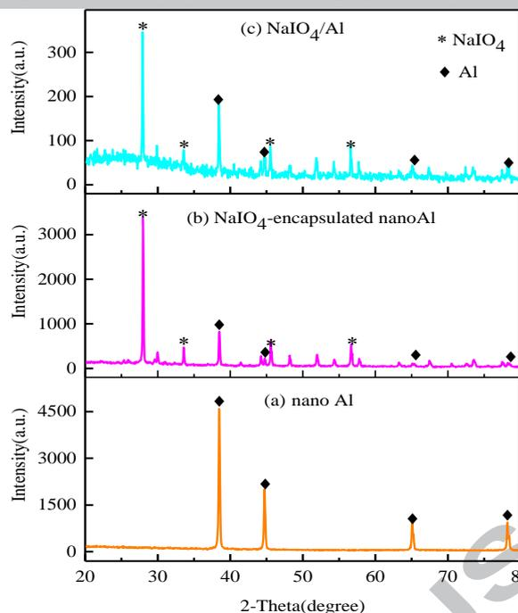
**Fig. 3.** XRD analysis for (a) nanoAl, (b) NaIO<sub>4</sub>-encapsulated nanoAl and (c) Al/NaIO<sub>4</sub> (by physical mixing).
