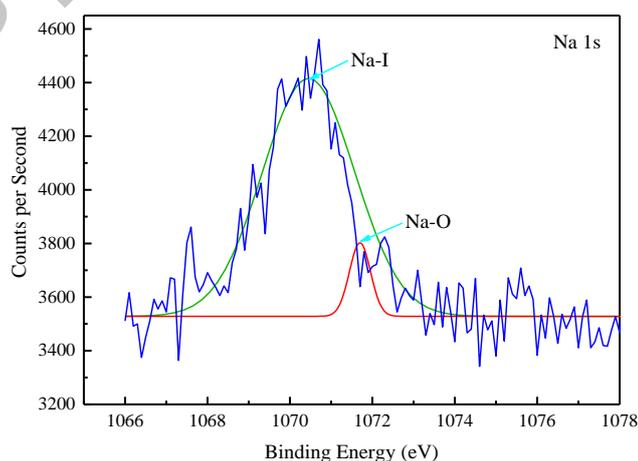
Fig. 6. XPS Na 1s spectra of reaction products of  $\text{NaIO}_4$ -encapsulated nanoAl.
