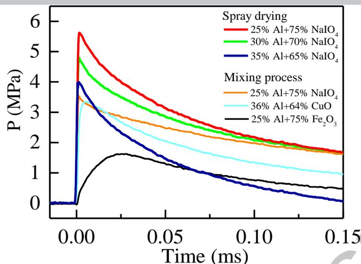
**Fig. 9.** Pressure trace of different proportions of  $\text{NaIO}_4$ -encapsulated nanoAl and Al/ $\text{NaIO}_4$ , Al/CuO and Al/ $\text{Fe}_2\text{O}_3$ .
