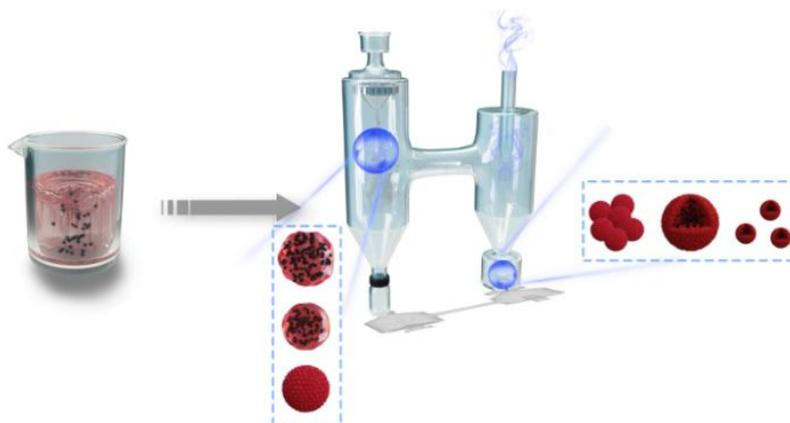
**Fig. 1.** Schematic illustration for the synthesis of  $\text{NaIO}_4$ -encapsulated nanoAl by continuous-flow spray drying.
