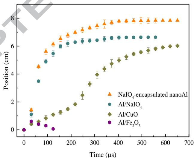
**Fig.8.** The position of the flame cone front as a function of time for  $\text{NaIO}_4$ -encapsulated nanoAl and  $\text{Al}/\text{NaIO}_4$ ,  $\text{Al}/\text{CuO}$  and  $\text{Al}/\text{Fe}_2\text{O}_3$ .
