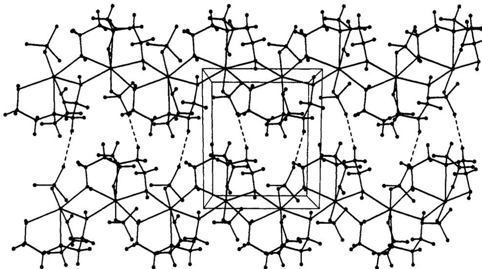
Figure 4. Molecular structure of 3. To more clearly illustrate interlayer hydrogen bonding, only one of the two chains in each layer traversing the unit cell is shown.
