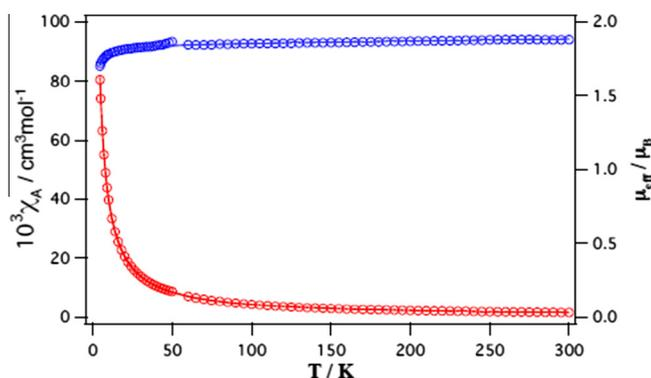
Fig. 3. Temperature dependence of magnetic susceptibilities (red circles) and effective magnetic moments (blue circles) for complex **1**. The solid lines represent the theoretical curves derived from Eq. (1) with the parameters of  $g = 2.13$  and  $J = -0.41 \text{ cm}^{-1}$ . (Color online.)
