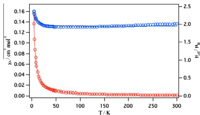
Fig. 4. Temperature dependence of magnetic susceptibilities (red circles) and effective magnetic moments (blue circles) for complex **2**. The solid lines represent the theoretical curves derived from Eq. (2) with the parameters of  $g = 2.20$  and  $J = 1.68 \text{ cm}^{-1}$ . (Color online.)
