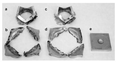
**Figure 7.** Witness plates from FGAN initiation experiments with polystyrene (a, c) and steel (b, d) base plates. The initiation was performed with plastic bonded explosive (a, b) and TACN (c, d). Inert material (sucrose) was used instead of FGAN in the case of (e)
