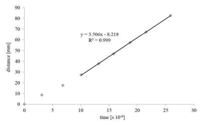
**Figure 8.** Detonation front tracking in steel confined TACN shows that the detonation velocity reached its steady value after 30 mm
