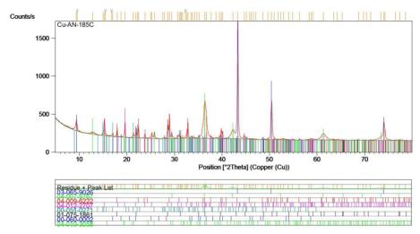
**Figure 3.** X-ray powder diffraction pattern of FGAN/Cu heated to 185 °C, using Cu Kα radiation ( $\lambda$ =1.5418 Å). The calculated peak positions of the reference patterns present are shown by coloured vertical bars
