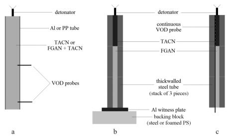
**Figure 1.** Schematic cross-sections of the detonation experiments: a) detonation velocity measurement; b) detonation capability of AN by TACN; c) detonation velocity of TACN under strong confinement
