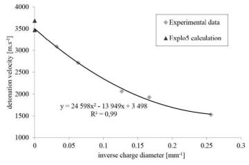
**Figure 6.** Determination of the theoretical maximum detonation velocity of tapped TACN
