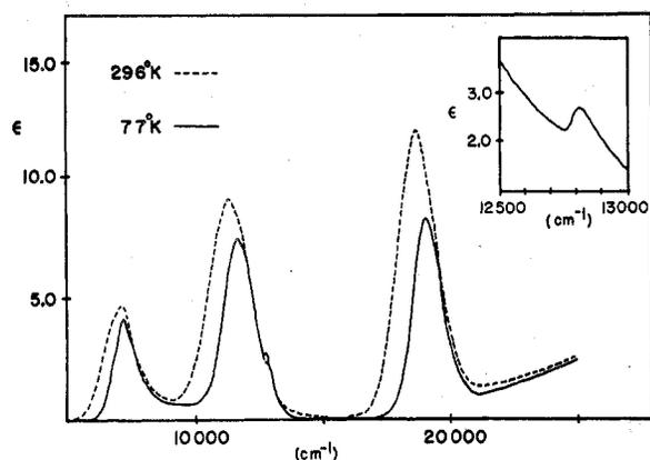
Figure 2. Ligand field spectrum of V(II) in CsCaCl<sub>3</sub> in the 5000–25 000-cm<sup>-1</sup> region. The inset in the upper right corner shows an expanded view of the high-energy portion of the second band at 77 K.
