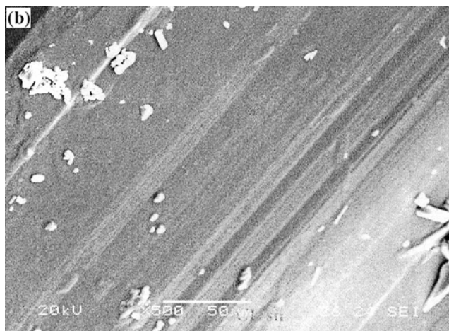
Fig. 7(b)—SEM micrograph of LARPCL single crystal showing microcrystallites
